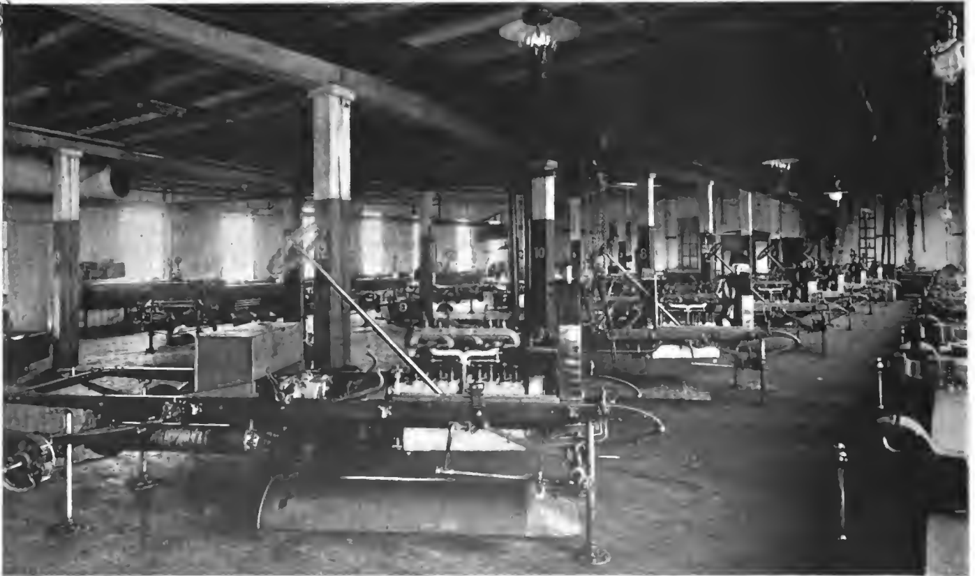
IN THE ASSEMBLING ROOM OF THE E. R. THOMAS DETROIT COMPANY, DETROIT, MICH.—THE ASSEMBLING STANDS WERE DESIGNED BY VICE-PRESIDENT F. E. COFFIN.—FOUR CARS PER DAY IS NOW THE REGULAR OUTPUT
